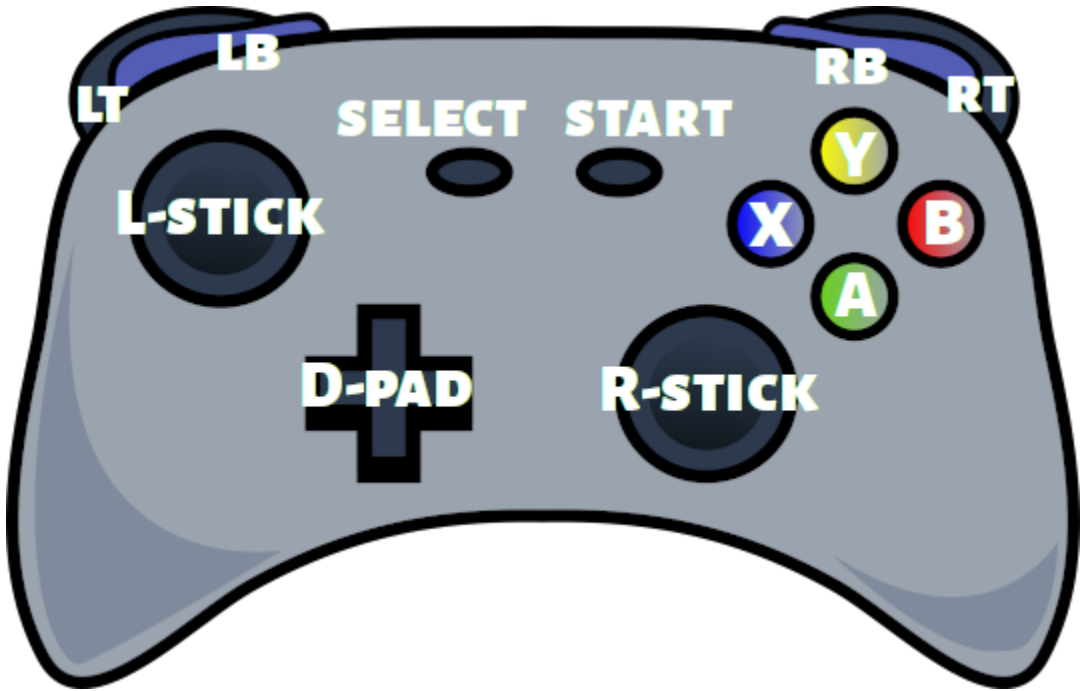
Fig. 44: Gamepad annotated with axes and buttons
