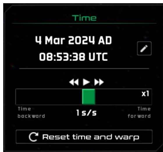
Fig. 27: The time pane displays the simulation date and time, along with controls to start and pause the time, and a slider to control the time warp (speed).
