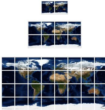
Fig. 87: An example of a virtual texture with 3 levels (0 to 2) for the Earth laid out as a quadtree. Note that the root (level 0, top), covers the whole area, while successive levels have equally-sized tiles that cover less and less area each. This VT has an aspect ratio of 2:1, so it has two root nodes at the top.
