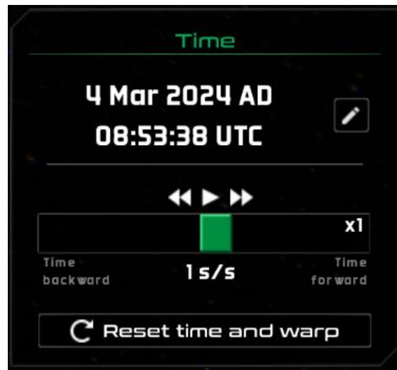
Fig. 26: The time pane displays the simulation date and time, along with controls to start and pause the time, and a slider to control the time warp (speed).
